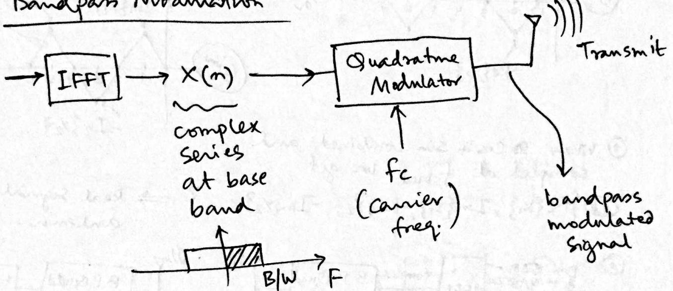
⑦ But note: Complex valued  $X_m$  needs to be transmitted as real valued signals from the antenna.
