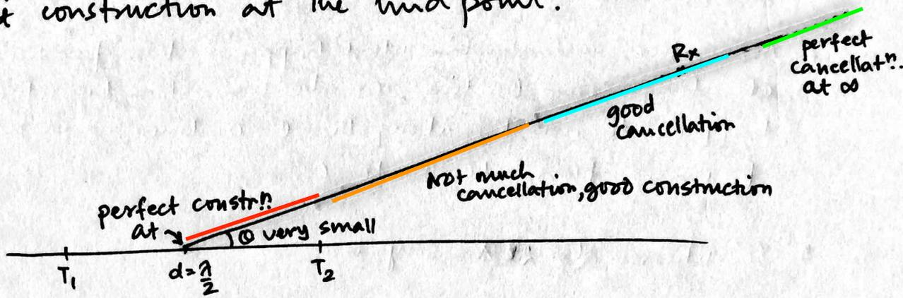
③ As  $\theta$  increases,  $d \cos \theta$  becomes smaller, so as in the graph shown earlier, the signal interaction now becomes closer to perfect construction. Thus around the bisection of  $(T_1, T_2)$ , the Rx experiences moderate to good signal construction.
